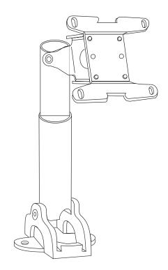
Typical Pedestal Type Mount with Swivel Bracket
